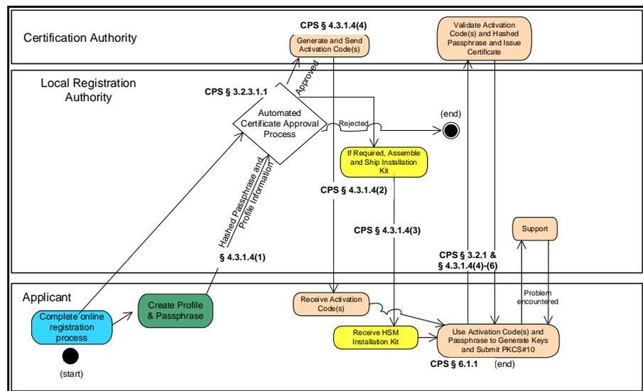
**Figure 5a: Activation Code-Account Password Process: Automated I&A**
